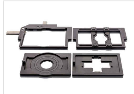
Various stage inserts let you use different cell culture vessels.
