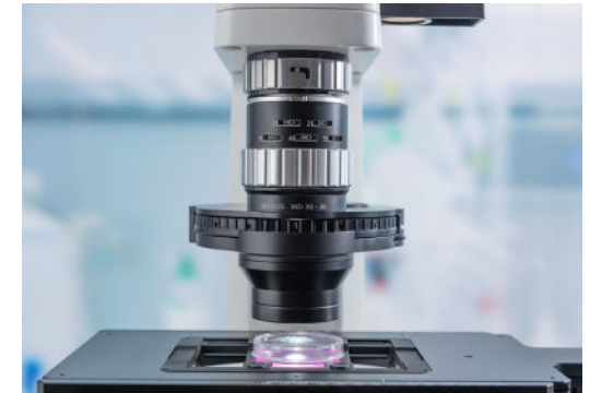
The LD condenser 0.55 offers a free working distance of up to 38 mm.
