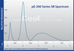
A microscope which is populated with a number of single band ("SB") filter sets will typically have DAPI excitation at 365 nm and a microscope with multi-band ("MB") filter(s) has excitation at 400 nm. The user can specify the configuration which is appropriate for their microscope.
