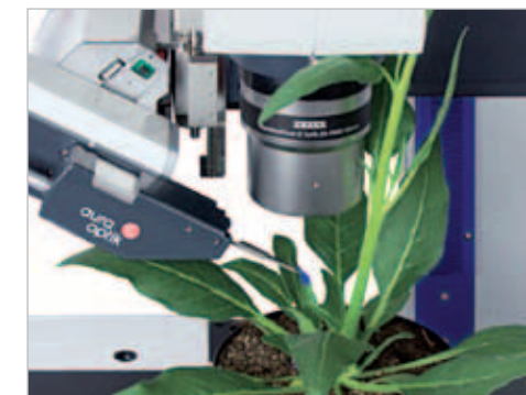
The large space between the objective and the stage can be used to handle all types of specimens. You can even isolate trichomes from tobacco plants if need be!
