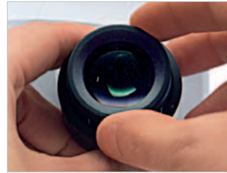
All eyepieces feature a diopter adjustment (foc.) so that they can be perfectly matched to every individual eye.
