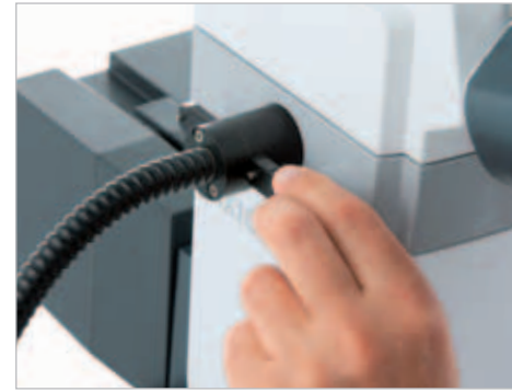
By changing the angle of the oblique reflected light, you can bring out textures and small steps on smooth surfaces – especially at high magnification levels.
