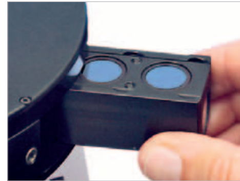
Changing filter cubes on PentaFluor S is easy. Just pull one out and slide another one in.
