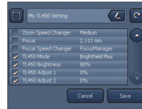
Use SYCOP 3 to store your entire device's configuration, including its transmitted light settings; then reproduce it as needed by simply pressing a button.
