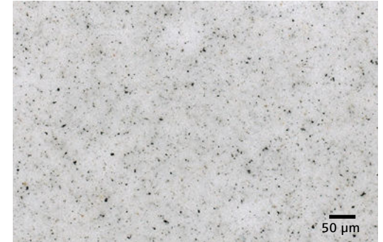
Particle analysis, brightfield, objective: EC Epiplan-NEOFLUAR 20×/0.5
