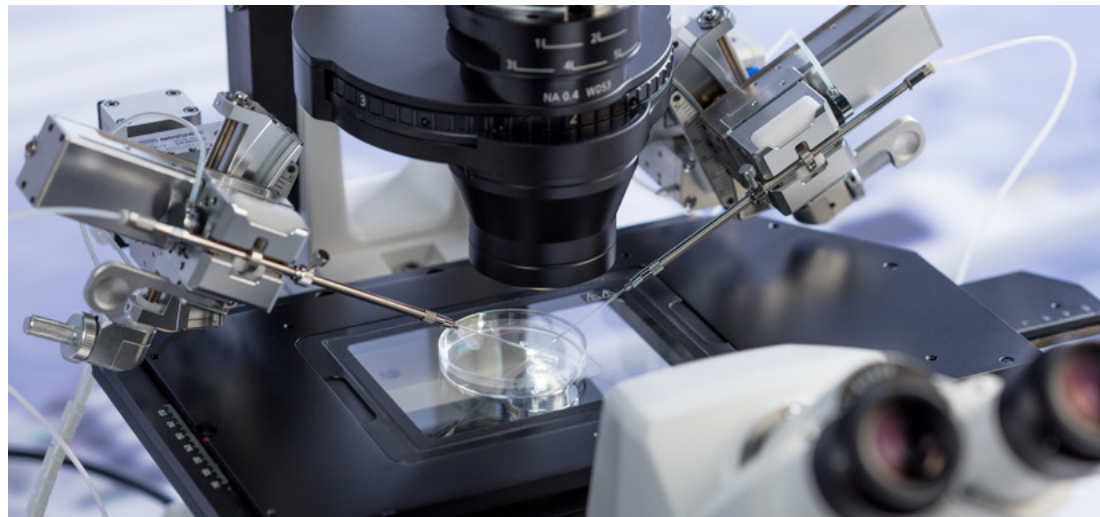
Axio Vert.A1 with manual stage combined with heating plate and micromanipulation setup
