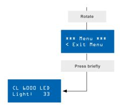
Rotate the incremental encoder (2) in the menu to access the menu item "Exit Menu". Briefly press the incremental encoder (2) to exit the menu and revert to regular operation mode.
