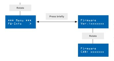
Rotate the incremental encoder (2) in the menu to access the menu item "FW Info" for firmware information. Briefly press the incremental encoder (2), and the information items will be shown in the display shortly one after another. Subsequently, the display will automatically revert to the menu item 'FW Info'. This menu item is provided for information only and cannot be used to set device parameters.
