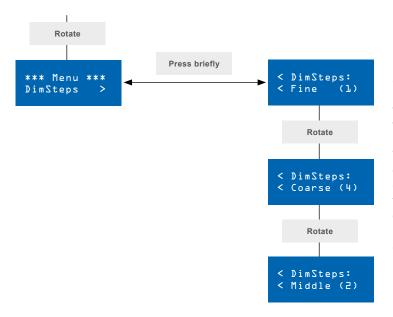
Rotate the incremental encoder (2) in the menu to access the menu item "DimSteps". Briefly press the incremental encoder (2) to access a sub-menu where the fineness of intensity steps can be adjusted. Rotate the encoder (2) to select between the settings 'coarse', 'medium" and 'fine'.
