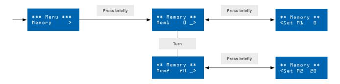
By turning the rotary encoder (2) in the submenu "Memory" you will access the subitem "Exit menu". By pressing the rotary encoder (2) again briefly you will leave the submenu "Memory".
