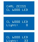
Display indication directly after switch-on. The display changes after a few seconds. (Also applicable to CL 9000 LED)
