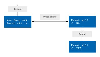
Rotate the incremental encoder (2) in the menu to access the menu item 'Reset all'. Briefly press the rotary encoder (2) to access a sub-menu where the factory settings of the device can be re-instated. The display shows the question 'Reset all?'. Rotate the incremental encoder to decide between 'NO' and 'YES' and briefly press the incremental encoder (2) to confirm your selection.
